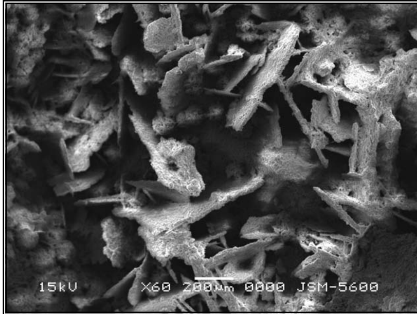
Sample S3: Secondary electron image (SEI) showed coarse-grained flaky crystals in the crack.
